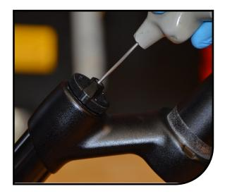
2 Remove the black compression knob, (2) detent balls, and (2) detent springs
