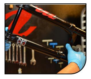
5 Insert 7cc of semi-bath into each casting leg. Once the semi-bath is in the legs, slide the casting the rest of the way onto the stanchion assembly.
