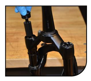
5 Using Manitou 24mm Flat Ground Socket and a torque wrench, rotate the compression damper top cap clockwise and tighten to 45-55 in lb [5.1-6.2 N m].
