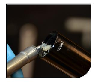
Install air spring assembly into stanchion. Rotating clockwise, start the end cap threads by hand to prevent cross-threading. Using a 22mm crow's foot and torque wrench, torque to 80-100 in lb [9.0-11.3 N m].
