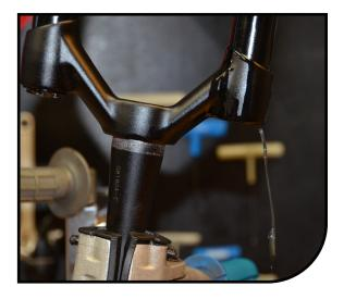
6 Invert the fork. Using a 22mm wrench, rotate the rebound damper end cap counter-clockwise until threads completely disengage from stanchion.
