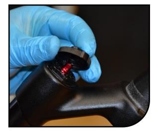
3 Using Manitou 24mm Flat Ground Socket, rotate compression damper top cap counter-clockwise until threads completely disengage from the stanchion
