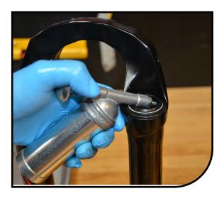
2 Tightly assemble shock pump fitting to comp rod end fitting. Inflate the air spring to 50 PSI. The air spring should not move during inflation. With the shock pump still attached, pull on the comp rod to full extension (you should feel some compression of the internal top-out bumper). Remove the shock pump. This process will ease casting installation.
