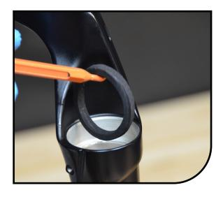
8 Remove springs from lip of dust seals. Using the Manitou 32mm Seal Press or large socket, press in the dust seals. Reinstall springs onto seals.
