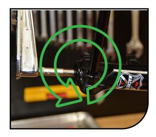
8 Using the Manitou 8mm Thin Wall Socket and torque wrench, turn the compression rod **counter-clockwise.** Torque to
