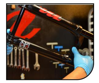
5 Insert 7cc of semi-bath into each casting leg. Once the semi-bath is in the legs, slide the casting the rest of the way onto the stanchion assembly.
