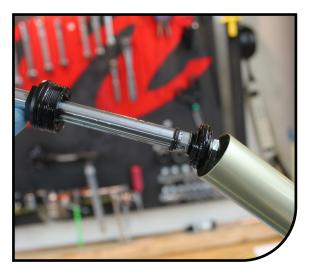
Install rebound damper assembly into stanchion. Rotating clockwise, start the end cap threads by hand to prevent cross-threading.
