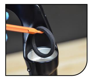
8 Remove springs from lip of dust seals. Using the Manitou 32mm Seal Press or large socket, press in the dust seals. Reinstall springs onto seals.
