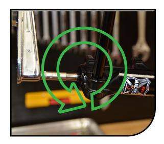
8 Using the Manitou 8mm Thin Wall Socket and torque wrench, turn the compression rod **counterclockwise.** Torque to 30-40 in Ibs [3,4-4,5 N m]. Do not overtighten, as doing so can damage the end of the rods.
