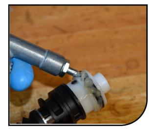
6 Add Slickoleum<sup>™</sup> grease to the stanchion threads before inserting the air spring assembly. Spread grease across entire thread surface.
