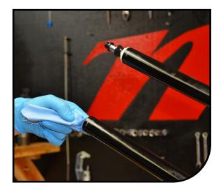
Liberally grease the piston quad seal and outer surface with Slickoleum<sup>™</sup> grease. Also add 3cc's of Slickoleum<sup>™</sup> grease to the top of the air piston.
