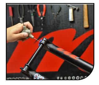
2 Insert an 8mm Hex wrench into the end of the rebound rod and rotate **clockwise**. The rebound end fitting will move toward the inside of the casting. Continue rotating until end fitting disengages completely from casting threads.
