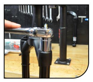
2 Invert the fork. Using a 22mm wrench, rotate the air spring end cap counter-clockwise until threads completely disengage from stanchion.
