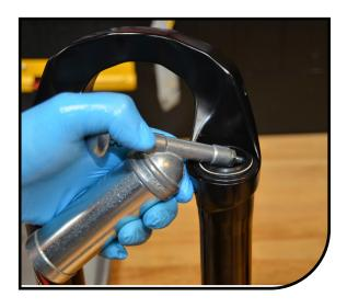
2 Tightly assemble shock pump fitting to comp rod end fitting. Inflate the air spring to 50 PSI. The air spring should not move during inflation. With the shock pump still attached, lightly pull the comp rod to full extension so that some compression of the internal top-out bumper can be felt. Remove the shock pump. This process will ease casting installation.
