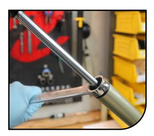
Invert the fork. Using a 22mm wrench, rotate the rebound damper end cap counter-clockwise until threads completely disengage from stanchion. Remove rebound damper from the fork. Clean the inside of the stanchion with isopropyl alcohol and a lint-free towel. Inspect the inside and outside of the stanchion for scratches and other damage. Inspect rebound damper for wear/damage and replace if necessary.
