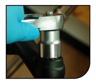
Invert the fork. Using a 22mm wrench, rotate the air spring end cap counter-clockwise until threads completely disengage from stanchion.
