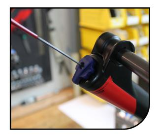
Insert an 8mm hex wrench into the end of the rebound damper rod and turn the rod **clockwise** until it is disengaged from the casting and can be pushed into the casting.
