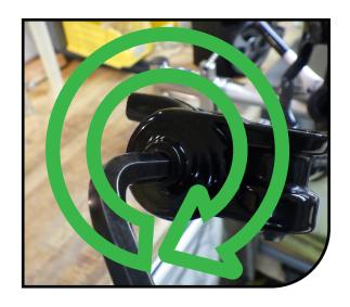
Use a 6mm hex wrench to remove the compression rod turn the rod **clockwise** until it is disengaged from the casting and can be pushed into the casting.
