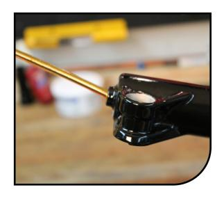
Using an 8mm hex wrench and torque wrench, tighten the rebound damper rod to 35–40 in lb [3.95–4.5 N m] by turning them **counter-clockwise.** Do not overtighten, doing so can damage the end of the rods.
