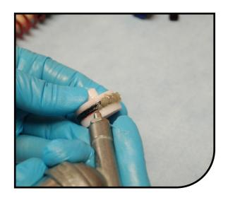
Add Slickoleum grease to upper stanchion threads before inserting the air piston. Spread grease across entire thread surface. Install air piston by pushing it past the upper stanchion threads. Piston height will be set automatically when air pressure is added in a later step.
