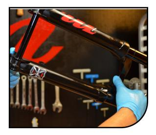
Insert 7cc's (7ml) of semi-bath into each casting leg. Once the semi-bath is in the legs, slide the casting the rest of the way onto the stanchion assembly.
