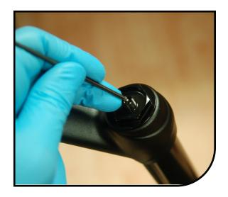
Using Manitou 24mm Flat Ground Socket, rotate air spring top cap counter-clockwise and remove when threads completely disengage from the stanchion.
