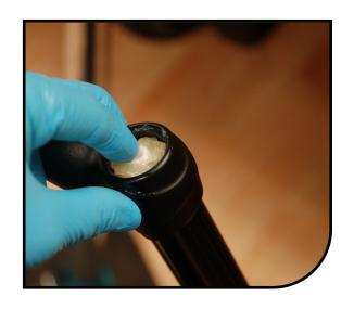
Add 3cc's of Slickoleum™ grease to the top of the air piston.
