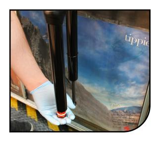
Inspect the air piston and piston seal for wear/damage and replace if necessary. Liberally grease the piston quad seal and outer surface with Slickoleum™ grease.
