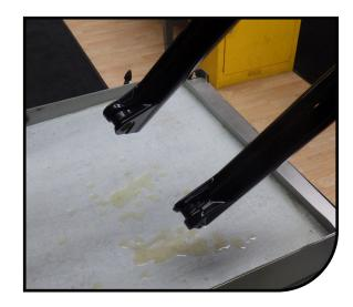
Using a downhill tire lever or similar 5 tool, gently pry the dust seals out of the casting.
