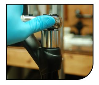
Install air spring assembly into stanchion. Rotating clockwise, start the end cap threads by hand to prevent cross-threading. Using a 22mm crow's foot and torque wrench, torque to 80-100 in lbs [9.0-11.3 N m].
