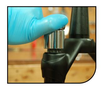
Remove Kwik Toggle compression damper assembly from the stanchion.
