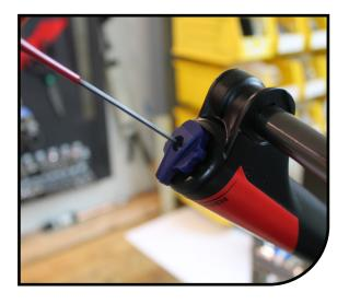
Using a 6mm hex wrench and torque wrench, tighten the compression rod to 35-40 in lbs [3.95-4.5 N m] by rotating counter-clockwise.
