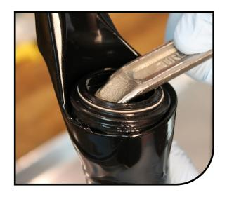
Remove old foam wiper rings. Apply 6 semi-bath fluid to the new foam wiper rings and install into fork casting.
