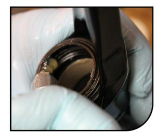
Tightly assemble shock pump fitting to air top cap. Inflate the air spring to 40-50 PSI.
