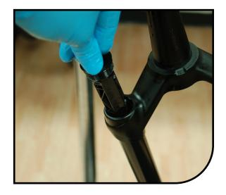
Rotating clockwise, use a torque wrench and a standard cassette lockring tool, such as Park Tool's FR-5.2, with the appropriate socket to torque the compression damper assembly to 45-55 in lbs [5.1-6.2 N m]
