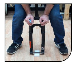
Pour additional 5wt fork oil into the damper leg until the oil height (space from the top of the damper leg to the top of the oil) is set at the proper level of **87mm**. An oil height setting tool used for motorcycle forks similar to the one pictured makes this job easier.
