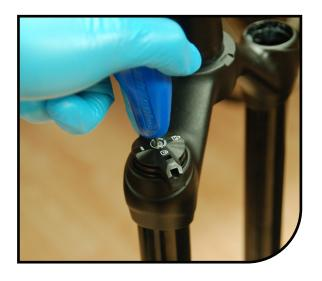
Use a standard cassette lockring tool, such as Park Tool FR-5.2, with the appropriate socket to rotate compression damper top cap counter-clockwise until threads completely disengage from the stanchion.
