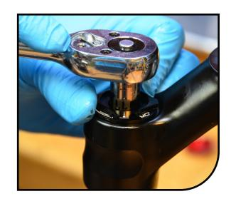
Remove the v-seal that was under the black "HI-SPEED" adjustment knob.
