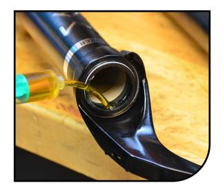
Make sure the spring shaft is fully 2 extended and air chamber is filled with air (60PSI).
