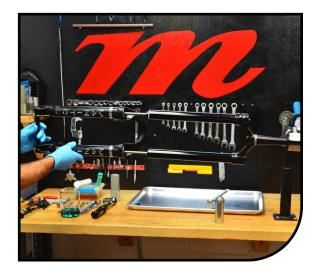
Insert 21cc of semi-bath (85-0022) into each casting leg. Once the semi-bath is in the legs slide the casting the rest of the way onto the stanchion assembly until the damper and spring shaft adapters pass thru the end of the casting. Some manual alignment may be needed.
