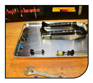
Liberally apply Slickoleum™ grease to the piston seal, outer piston surface, and spring shaft. Add 3cc's of Slickoleum™ grease to the top of the air piston.
