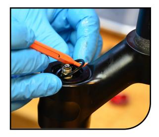
Use a standard cassette tool and 1" 5 socket to unthread the damper topcap from the stanchion.
