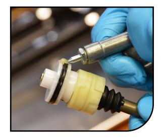
Add Slickoleum™ grease to the 8 stanchion threads before inserting the air spring assembly. Spread grease across entire thread surface.
