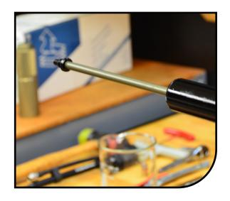
Fully extend the damper shaft.
