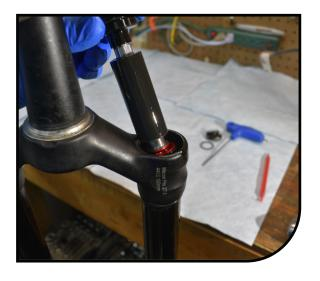
Clean the adjuster knobs with isopropyl and replace v-seal into damper top cap. Install the black VTT adjustment knob onto adjuster hex, being sure the knob can fully rotate without contacting the crown. With a 2mm hex, thread on the screw and torque to 4-6 in-lb [0.5-0.7 Nm] Note: Be sure to hold the knob still while installing the
