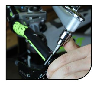
To adjust lever reach, use the dial to turn the lever reach adjust screw. Turning it in the "-" direction will move the lever in. Turning it in the "+" direction will move the lever out. Do not force the screw beyond its limits.
