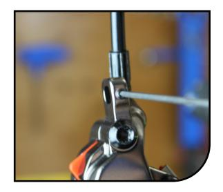
Place the caliper feet onto the mounting surface and thread the mount bolts (with washers) into the mount leaving the caliper loose.
