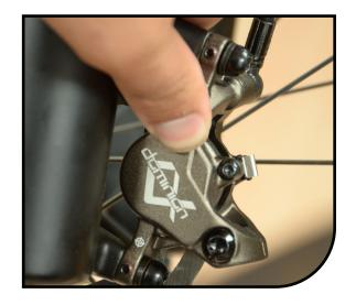
Snug the mount bolts using the 5 5mm hex tool while keeping the outer pad against the disc.
