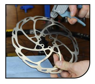
Place the disc on the hub mounting surface. Be sure that the arrow on the disc is pointing in the same direction of the forward wheel rotation.
