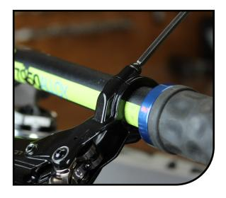
Once you have set the master 3 cylinder in the final desired position on your handlebars, tighten down the top mount bolt. Torque to 30±5 in lbs  $(3.39\pm0.56 \text{ N m})$ . Next tighten down the other bolt to a torque of  $30\pm5$  in-lb  $(3.39\pm0.56$  N m).
