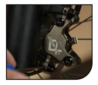
Torque the lower mount bolt (A) to 80±5 in lbs (9.0±0.5 N m). (the upper adjuster screw keeps the caliper from rotating out of alignment). Torque the upper mount bolt (B) to 80±5 in lbs (9.0±0.5 N m).
