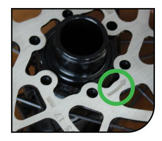
Using a T25 Torx driver, install, tighten, and torque the disc screws to 50±5 in lbs (5.65±0.56 N m), in a star pattern sequence.
