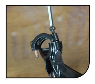
\*Optional, install either Shimano™ or SRAM™ PeaceMaker clamp. Torque bolts to 30±5 in lbs (3.39±0.56 N m).
