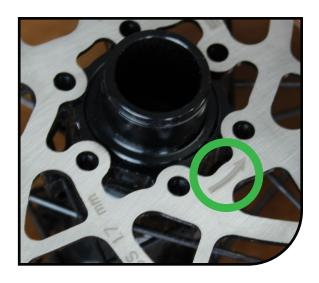
Using a T25 Torx driver, install, tighten, and torque the disc screws to 50±5 in lbs (5.65±0.56 N m), in a star pattern sequence.
