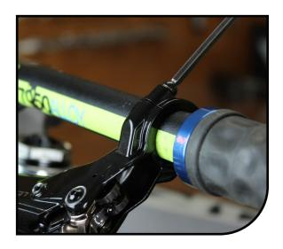
Once you have set the master cylinder in the final desired position on your handlebars, tighten down the top mount bolt. Torque to 30±5 in lbs (3.39±0.56 N m). Next tighten down the other bolt to a torque of 30±5 in-lb (3.39±0.56 N m).
