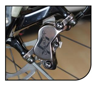
Using the 2mm hex tool, turn the adjuster screws clockwise until they contact the mount bolts.
