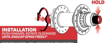
BEFORE INSTALLED ON BIKE, A SMALL AMOUNT OF SIDE-TO-SIDE PLAY IS NORMAL
