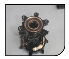
Install the spacer, lightly grease and press in the driver side (DS) bearing.
