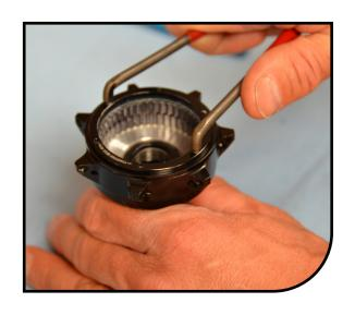
Using the 90 Degree pick tool pry out the top rachet ring.
