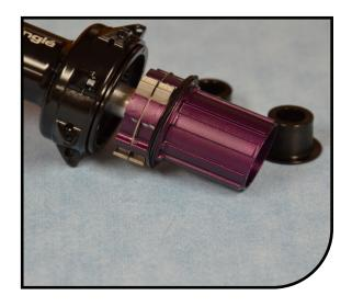
Remove the crush tube.
