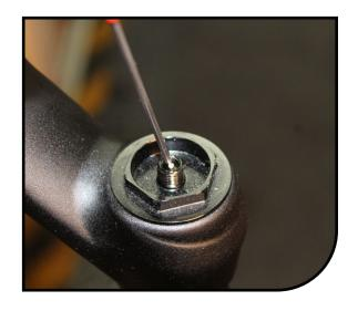
Remove air cap using a 20mm socket.
