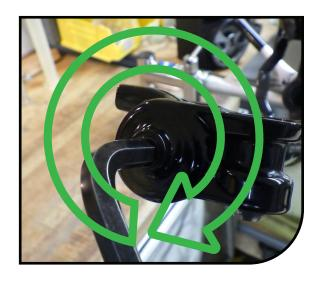
3 Use a 12mm wrench to remove the compression rod bolt.
