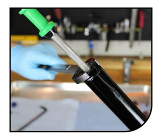
Remove compression rod assembly from the stanchion. Clean the assembly and re-grease.
