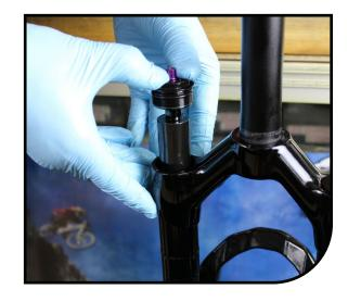
Install the ABS+ damper using a 24mm socket and torque wrench, tighten the damper to 60–80 in lbs [6.8–9.0 NM].
