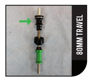
Liberally grease the piston seal and outer surface with Slickoleum™ grease
