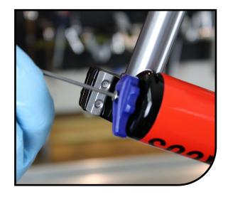
Install compression rod bolt. It helps to have at least 30-50PSI in the air chamber when tightening down the bolt to the proper torque. Use a 12mm socket and torque wrench and tighten to 45–55 in lb [5.1–6.2 N m].
