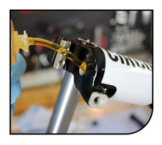
Using an 8mm hex wrench tighten the rebound damper rod and air spring assembly to 35–40in lbs [3.95–4.5 Nm] by turning them **counter-clockwise.** Do not overtighten, doing so can damage the end of the rods.
