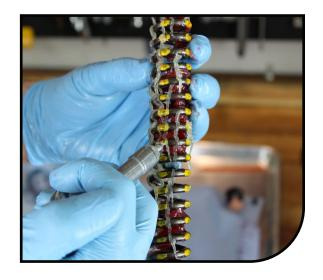
Insert the compression spring and install air cap onto stanchion. Tighten to 60-80 in lbs. [6.8-9.0 NM].
