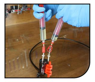
14 Add slight positive pressure to the MC and remove the syringe from the master cylinder and install the bleed screw using your T10 torx and torque to 12 in lbs [1.5N m]. Clean your MC and caliper with isopropyl alcohol and check the brake for proper function.
