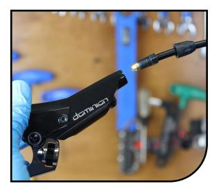
5 Using an 8mm crows foot, torque the hose nut to  $70 \pm 5$  in lbs [7.9±0.5 N m]
