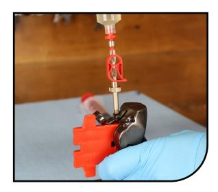
5 Fill second syringe 1/4 full of DOT 5.1 fluid, eliminate all air from syringe, and close hose clip. Remove the MC bleed screw using a T10 Torx wrench and attach to the MC bleeder.
