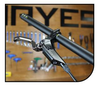
2 Using a 3mm hex key remove the KingPin from your caliper and remove the pads. Push the pistons back fully. Make sure the caliper is vertical when bleeding.
