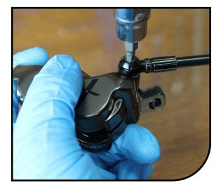
Reattach the hose to the caliper and bleed the system.
