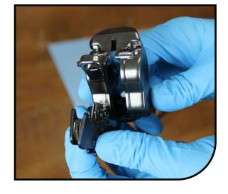
3 Fill space in caliper with dummy pads and bleed block or something else. If nothing is available then be careful during bleed not to advance the pistons.
