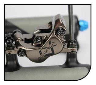
2 If there is nothing wrong with the hose and the hose fitting, completely remove the caliper hose assembly using a 3mm hex wrench.
