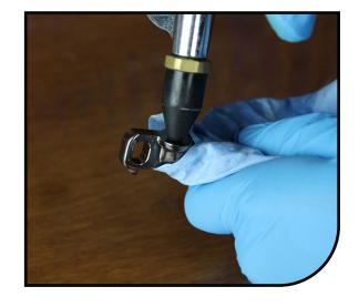
8 Clean all of the parts. Then rinse each part with mild soap and water. Be sure to clean the caliper through all of the holes.
