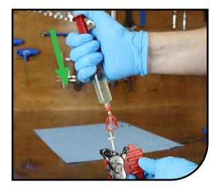
Push DOT 5.1 fluid from caliper 8 syringe to MC syringe while flicking the lever several times, then return.
