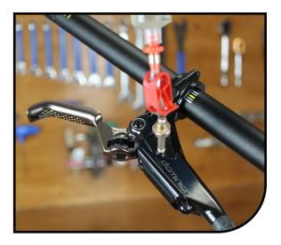
6 Open both syringe hose clips and pull a small vacuum at the caliper syringe to pull any air that was introduced.
