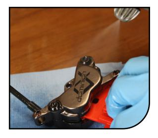
15 Re-install your pads and tighten KingPin using 3mm hex, torque to 30 in lbs [3.5 N m]
