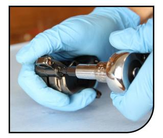
4 Take the transfer port O-ring out and inspect it for any cuts or debris. This O-ring may be reused when the caliper is put back together.
