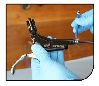
2 Pull the hose out of the MC. There will be residual fluid in the master cylinder body. Be careful to avoid spilling the fluid.
