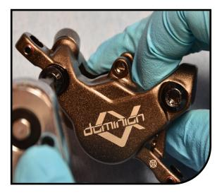
Reattach the hose to the caliper. Torque the Bajo bolt to 60 in lbs +/- 5 in lbs [6.78 N m +/-0.5 N m]
