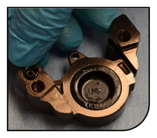
2 Put the two caliper haves together and install the bridge bolts. Torque the bridge bolts to 170 in lbs +/- 5 in lbs [19.2 N m +/-0.5 N m]
