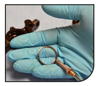
2 Carefully push the square seal into its seal groove – making sure that the seal is worked into the groove all of the way around and that it is pushed all of the way to the back of the seal groove.
