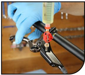
8 Push DOT 5.1 fluid from caliper syringe to MC syringe while flicking the lever several times, then return.
